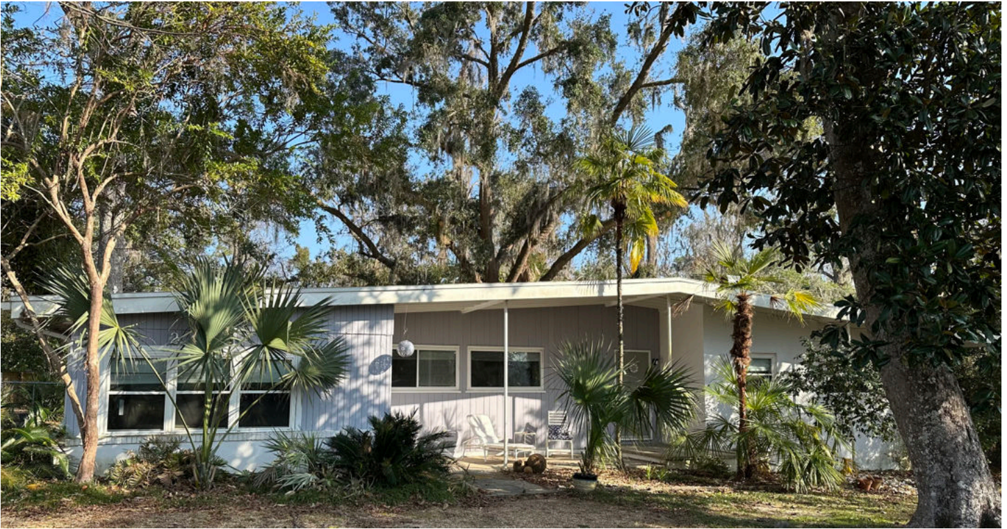
Low pitch roof and skinny tubular steel Lally columns provide structural support on porch. Often seen as supports on carports also.
